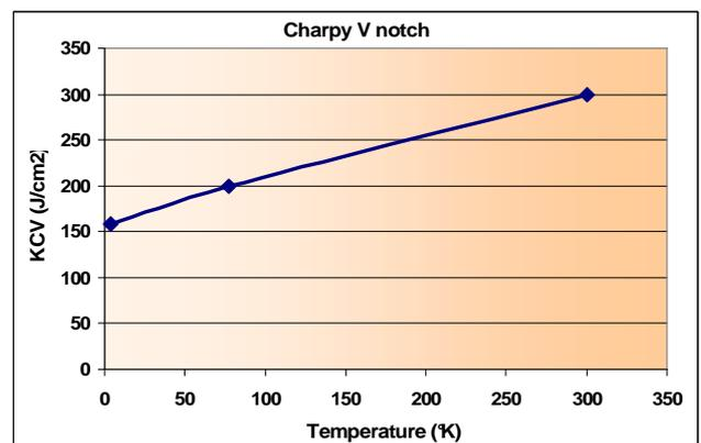
Thanks to its fully austenitic structure at all temperatures, Invar® M93 has good ductility and toughness and consequently, offers good formability (deep drawing, folding, bending, etc...) without any risk of embrittlement when at cryogenic temperature, even in the case of high deformation rate made at room temperature. The austenitic structure also makes the welding operations easier during tubes fabrication and tubes assembly.
